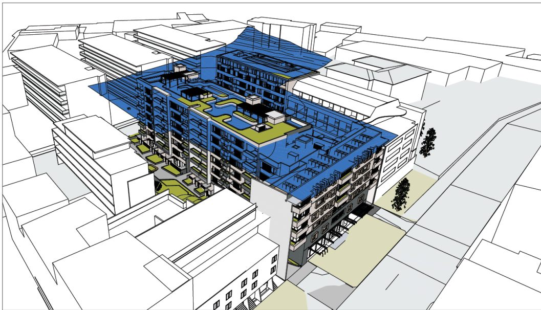
Figure 1 Encroachments to the 22m height standard (Source: Coffee Parker)
